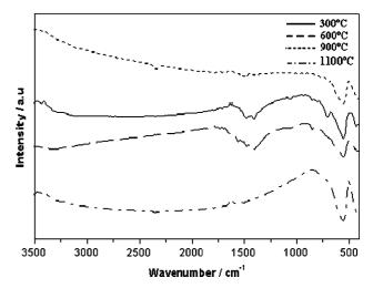
Fig. 3. Infrared spectroscopy of LaFeO  $_{\!3}$  calcinated at 300, 600, 900 and 1100  $^{\circ}\text{C}.$
