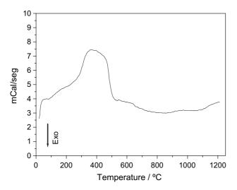
Fig. 2. DTA of LaFeO<sub>3</sub> precursor resin calcinated at 300 °C.
