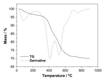
Fig. 1. Thermogravimetric curve of LaFeO<sub>3</sub> precursor resin calcinated at 300 °C
