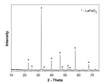
Fig. 4. X-ray diffraction pattern of LaFeO<sub>3</sub> calcinated at 900 °C.
