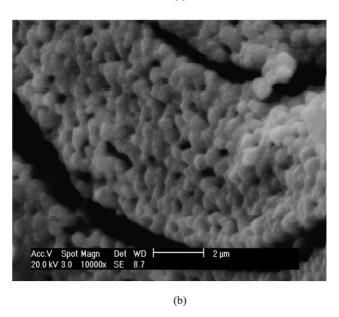
Fig. 6. SEM images of powders calcinated at (a) 900  $^{\circ} C$  and (b) 1100  $^{\circ} C$  for 4 h.
