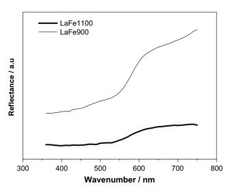
Fig. 5. UV-visible pattern of LaFeO<sub>3</sub> calcinated at 900 and 1100 °C.
